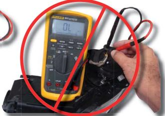
Do not insert fingers or DVOM into the HID module output connection when the headlights are on.
