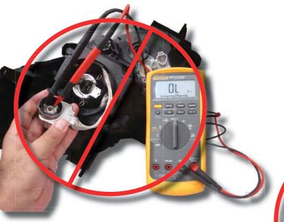
Do not insert fingers or DVOM into HID bulb socket when the headlights are on.
